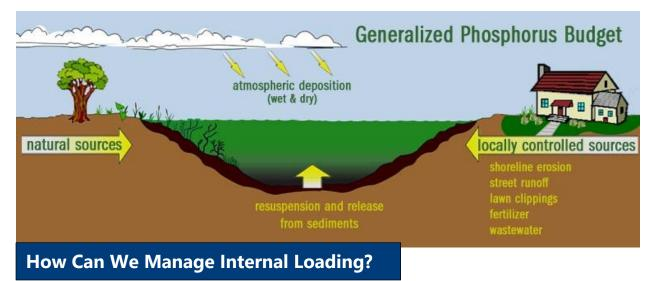
Aluminum sulfate (alum) is the most common method used to control phosphorus release from the lake bottom sediments (internal loading). Alum is applied to lakes using specialized equipment and barges that ensure the precise
