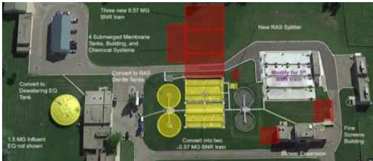
Figure 4-8. Alternative 3: MBR without Primary Treatment site layout
