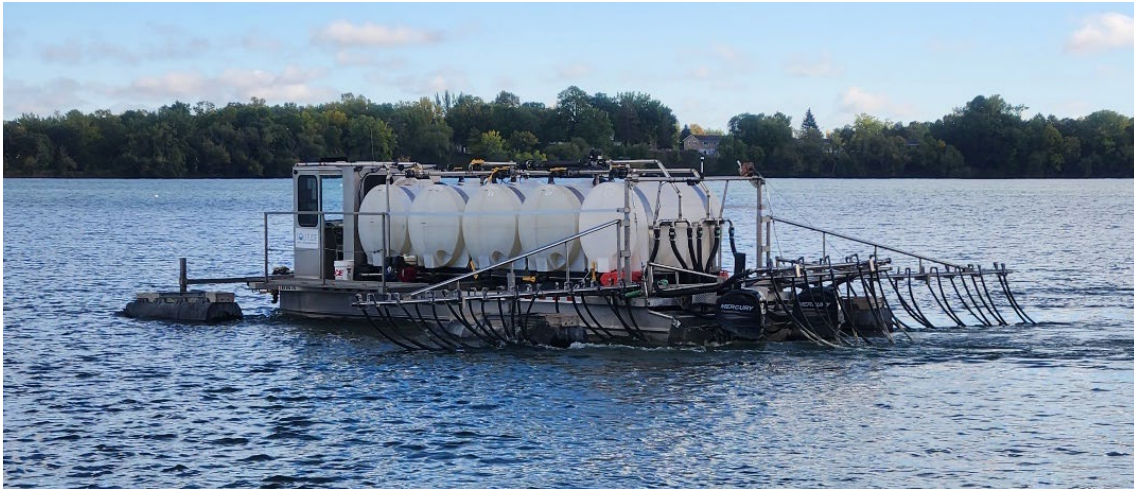
Figure ES-1. Alum application barge in Lake Agnes (September 22, 2022).
