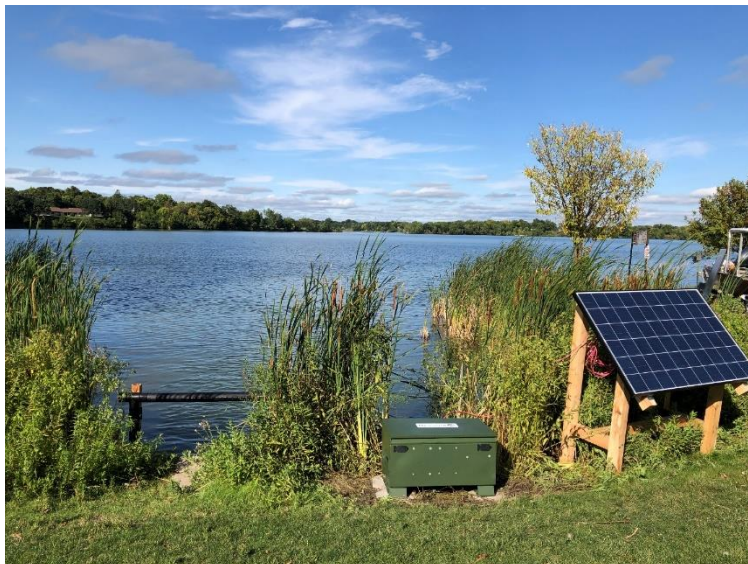
Figure 7. Stationary passive integrated transponder tag passage detection system at the Lake Agnes inlet.
