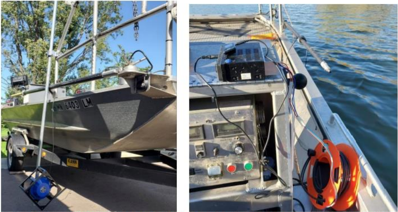
Figure 4: Representation of speaker mounted to boat on left with amplification and sound control on right.
