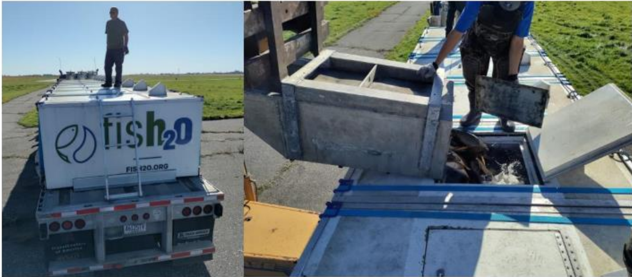
Figure 10: Fish20 truck preloaded with water and oxygen to keep carp alive in travel. On right, each fish box was dumped into one of the 10 tanks on the semi.
